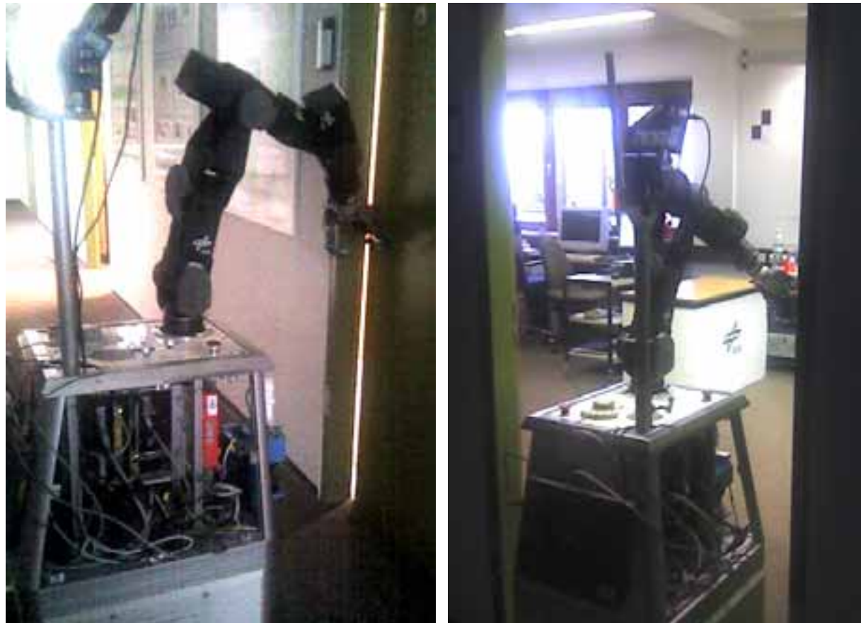
Figure C.28. Dexterous arm on mobile base, opening door (left), robot passing through doorway (right).
