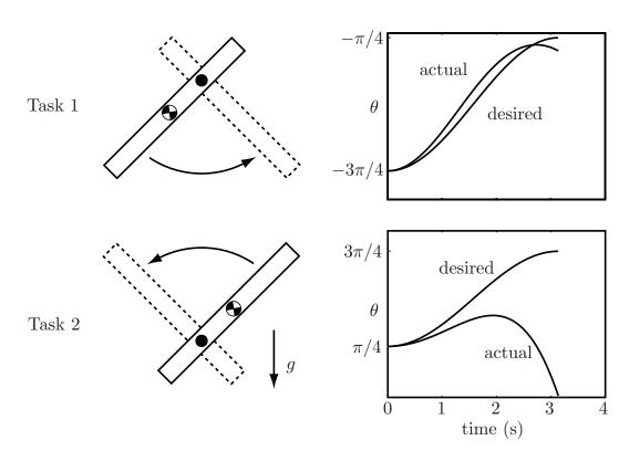
Figure 11.17: Results of feedforward control with an incorrect model:  $\tilde{r} = 0.08$  m, but r = 0.1 m. The desired trajectory in Task 1 is  $\theta_d(t) = -\pi/2 - (\pi/4)\cos(t)$  for  $0 \le t \le \pi$ . The desired trajectory for Task 2 is  $\theta_d(t) = \pi/2 - (\pi/4)\cos(t)$ ,  $0 \le t \le \pi$ .
