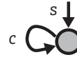
FIGURE 1.13: The dynamics of a single activation variable, illustrated by a circle filled in gray, is represented in the manner of neural networks. Excitatory external input, s , is indicated by an incoming arrow. Self-excitatory neural interaction is illustrated by a single recurrent loop ending in an arrow. The strength of that input is modulated by the parameter, c .
